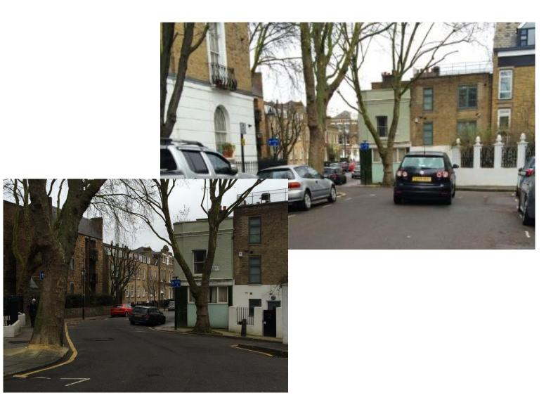
Narrowing of road leaves little room for contraflow cycles and oncoming traffic Double bend in road forces all traffic into centre, with risk to oncoming contraflow cyclists
