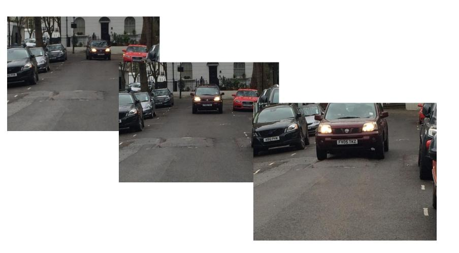
Cycle contraflow signs high and difficult to spot, Tree position occludes left hand sign from view
