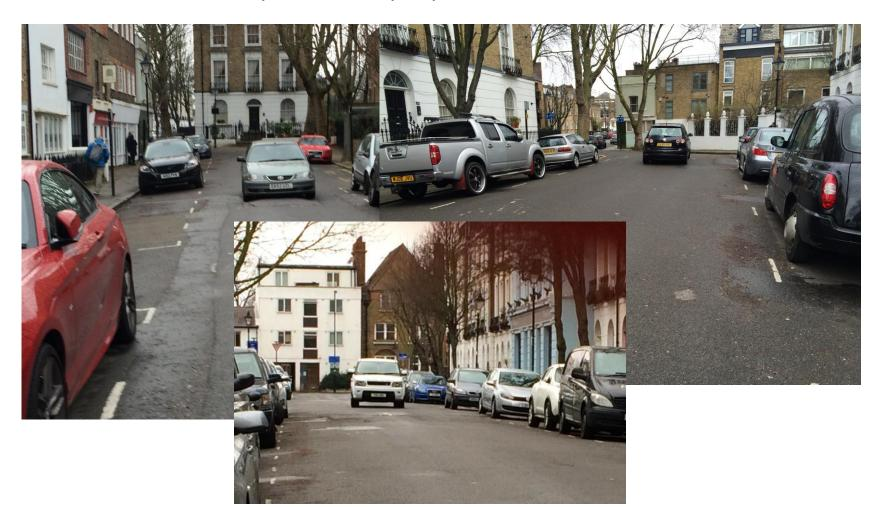
Motor vehicles move to centre of road to straddle the speed bumps: Both the two way and one way / cycle contraflow sections
